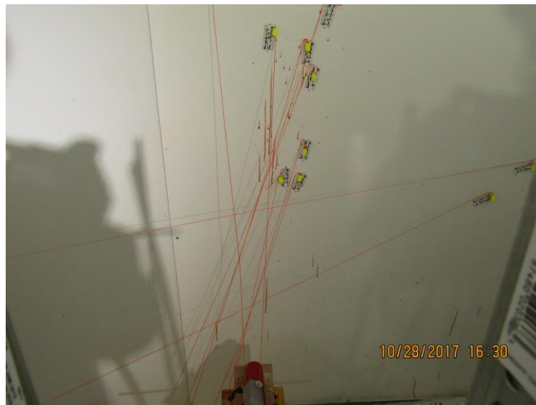
Figure 101. Simulation 3.4 string method construction.
